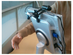
Figure 5. TOF depth camera on the stationary display setup
